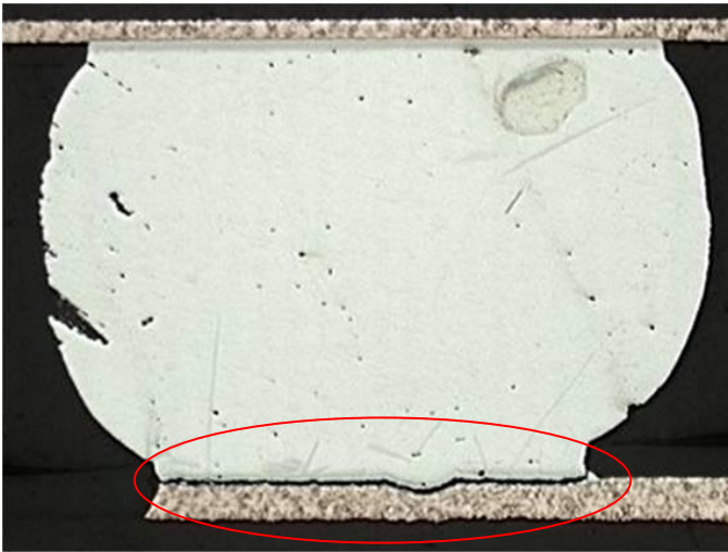
Fig. 4: 100% Fracture of BGA Solder Bump on Outer Row.
